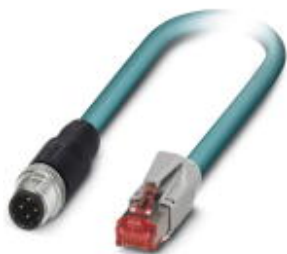
Assembled Ethernet cable, CAT5e, shielded, 2-pair, 26 AWG stranded (7-wire), RAL 5021 (water blue), M12 plug to RJ45 plug/IP20, line, length: 6 m
