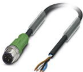
Sensor/actuator cable, 4-position, PUR halogen-free, black-gray RAL 7021, Plug straight M12, A-coded, on free cable end, cable length: 1.5 m, Without PATGs
