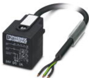
Sensor/actuator cable, 3-position, PUR halogen-free, black RAL 9005, free cable end, on Valve connector A, with 1 LED, connected with Damping diode, cable length: 3 m
