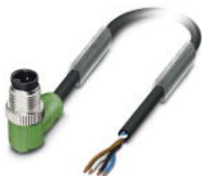
Sensor/actuator cable, 4-pos., PUR, halogen free, black-gray RAL 7021, angled M12 plug, D-coded, to free cable end, cable length: 0.3 m
