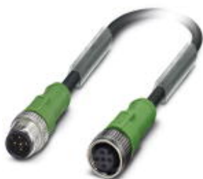
Sensor/actuator cable, 5-position, PUR halogen-free, black-gray RAL 7021, Plug straight M12, A-coded, on Socket straight M12, A-coded, cable length: 10 m
