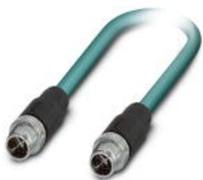
Assembled Ethernet cable, shielded, 4-pair, 26 AWG stranded (7-wire), RAL 5021 (water blue), M12 plug to M12 plug, SPEEDCON, length 10.0 m
