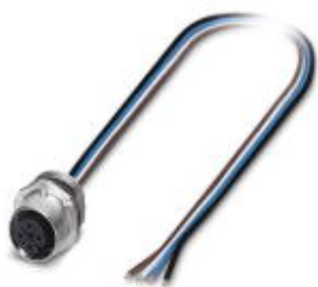
Sensor/actuator flush-type socket, 4-pos., M12 SPEEDCON, A-coded, front/screw mounting with M16 thread, with 1.5 m TPE litz wire, 4 x 0.34 mm 2
