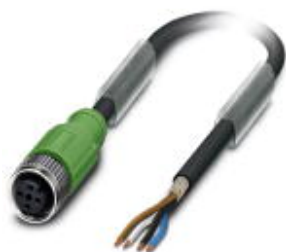
Sensor/actuator cable, 4-position, PUR halogen-free, black-gray RAL 7021, shielded, free cable end, on Socket straight M12 / IP67, coding: A, cable length: 1.1 m, Socket is 8-pos.
