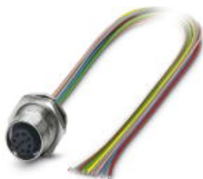
Sensor/actuator flush-type socket, 8-pos., M12 SPEEDCON, rear/screw mounting with Pg9 thread, with 2.0 m TPE litz wire, 8 x 0.34 mm 2
