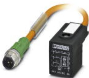
Sensor/actuator cable, 3-position, PUR halogen-free, irradiated, orange RAL 2003, Plug straight M12, A-coded, on Valve connector B (10 mm), with 1 LED, connected with Z diode, cable length: 1.5 m
