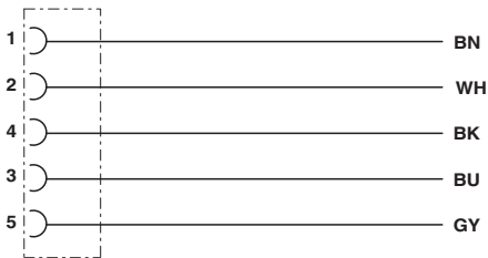
Contact assignment of the M12 socket
