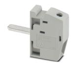
Panel feed-through terminal block, connection method: Screw connection with tension sleeve, Screw connection with tension sleeve, number of positions: 1, load current: 57 A, cross section: 0.5 mm² - 16 mm², connection direction of the conductor to plug-in direction: 0 °, width: 10.1 mm, color: white
