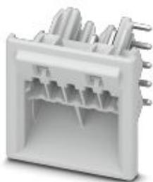
PCB headers, color: light gray, nominal current: 8 A, rated voltage (III/2): 150 V, contact surface: Tin, type of contact: Male connector, Number of potentials: 5, Number of rows: 1, Number of positions per row: 5, number of connections: 5, product range: ICC25-H/..R, pitch: 3.5 mm, mounting: Wave soldering, pin layout: Linear pinning, solder pin [P]: 2.8 mm, Locking: Snap-in locking, Product with pin output on right side
