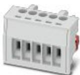
PCB connector, color: light gray, contact surface: Tin, Number of potentials: 5, Number of positions per row: 5, number of connections: 5, product range: ICC..-PSC1,5/..-3,5, pitch: 3.5 mm
