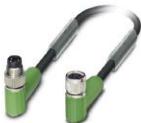
Sensor/actuator cable, 4-position, PUR halogen-free, black-gray RAL 7021, shielded, Plug angled M8, on Socket angled M8, cable length: 0.5 m
