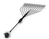
M17 series pre-assembled FO socket assembly: 24-position M17 socket, LC-Duplex on the other end, 0.6 m long, multi-mode fiberglass G62.5/125um OM1, IP67 degree of protection after being inserted, fixed installation for indoor use
