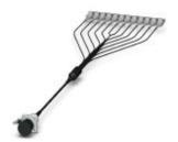
M17 series pre-assembled FO socket assembly: 24-position M17 socket, LC-Duplex on the other end, 1 m long, multi-mode fiberglass G62.5/125um OM1, IP67 degree of protection after being inserted, fixed installation for indoor use
