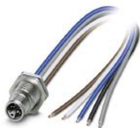
Flush-type connector, Power, 5-position, Plug, M12, L - Power, Rear mounting, M16 x 1.5, Individual wires, cable length: 0.5 m, 2.50 mm², PEX litz wire
