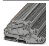
Multi-level terminal block, connection method: Push-in connection, cross section: 0.14 mm² - 1.5 mm², AWG: 26 - 14, width: 3.5 mm, color: gray, mounting type: NS 35/7,5
