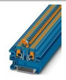
Knife disconnect terminal block, nom. voltage: 400 V, nominal current: 20 A, connection method: Pushin connection, cross section: 0.14 mm<sup>2</sup> - 4 mm<sup>2</sup>, AWG: 26 - 12, length: 62 mm, width: 5.2 mm, color: blue, mounting: NS 35/7,5, NS 35/15, nom. voltage: 400 V
