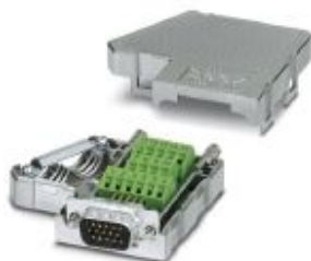
D-SUB connector, 15-pos, male connector, two 35° cable entries, universal type for all systems, pin assignment: 1, 2, 3, ..., 14, 15 to screw connection terminal block
