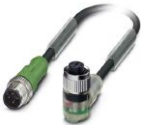
Sensor/actuator cable, 4-position, Variable cable type, Plug straight M12, coding: A, on Socket angled M12, coding: A, with 3 LEDs, cable length: Free input (0.2 ... 40.0 m)
