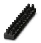
Polypropylene Europe terminal strip, black, for connecting solid conductors and stranded conductors with and without ferrules with a cross section of 1.5 to 16 mm<sup>2</sup>
