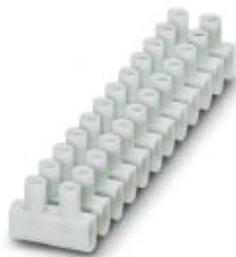
Polypropylene Europe terminal strip, white, for connecting solid conductors and stranded conductors with and without ferrules with a cross section of 1 to 10 mm<sup>2</sup>
