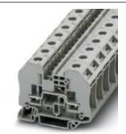
Thermoelectric voltage terminal block with bolt connection technology, cross section: 0.1 - 6 mm², AWG: 26 - 10, width: 16.3 mm, color: gray
