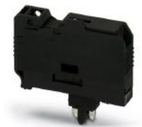
Fuse plug, nominal current: 10 A, width: 8.2 mm, fuse type: G / 6,3 x 32, color: black
