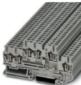
Double-level spring-cage terminal block, connection method: Spring-cage connection, cross section: 0.08 mm 2 - 4 mm 2 , AWG: 28 - 12, width: 5.2 mm, color: gray, mounting type: NS 35/7,5, NS 35/15
