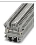
Feed-through terminal block, nom. voltage: 250 V, nominal current: 24 A, connection method: Screw connection, number of connections: 3, number of positions: 1, cross section: 0.2 mm² - 4 mm², AWG: 24 - 12, width: 5.08 mm, color: gray, mounting type: NS 32, NS 35/15, NS 35/7,5
