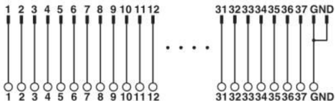
Connection scheme VIP-2/SC/D37SUB/M
