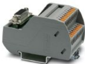
VARIOFACE module, with psh-in connection and D-subminiature socket strip, for mounting on NS 35 rails, with LED, 15-pos.
