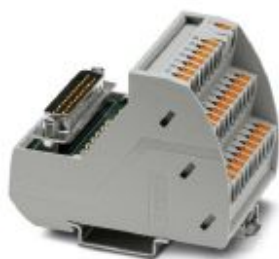
VARIOFACE module, with push-in connections and D-SUB miniature pin strip, for mounting on NS 35 rails, with LED, 25-pos.
