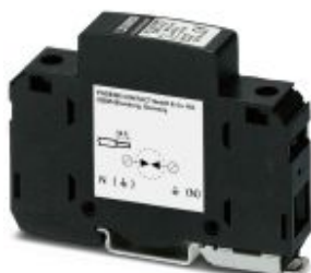
Lightning current arrester with encapsulated N-PE spark gap and ignition electronics, 1-channel. Voltage protection level: 4 kV Housing width: 17.5 mm (1 pitch)
