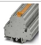
Knife disconnect terminal block, With test socket screws for insertion of test plugs, nom. voltage: 400 V, nominal current: 26 A, connection method: Screw connection, cross section: 0.2 mm² - 4 mm², AWG: 24 - 12, length: 80 mm, width: 6 mm, color: gray, mounting: NS 35/7,5, NS 35/15, NS 32
