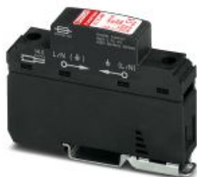
Type 1 / Class I / B arrester (lightning current arrester) with arc chopping spark gap, 1-channel. Housing width: 17.5 mm (1 Div.)
