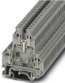
Component terminal block, with integrated diode, connection method: Screw connection, cross section: 0.2 mm 2 - 4 mm 2 , AWG: 24 - 12, width: 6.2 mm, color: gray, mounting type: NS 35/7,5, NS 35/15, NS 32
