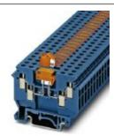
Feed-through terminal block, nom. voltage: 630 V, nominal current: 16 A, connection method: Screw connection, cross section: 0.2 mm² - 6 mm², AWG: 24 - 10, length: 63.5 mm, width: 6.2 mm, color: blue, mounting: NS 32, NS 35/7,5, NS 35/15
