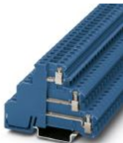
Sensor/actuator terminal block, connection method: Screw connection, cross section: 0.2 mm 2 - 4 mm 2 , AWG: 24 - 12, width: 6.2 mm, color: blue, mounting type: NS 35/7,5, NS 35/15
