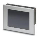
Touch panel with 14.5 cm/5.7" TFT active-display (analog resistive (polyester)), 320 x 240 pixel(s) (QVGA), 65536 colors, Arm9™, 200 MHz, 2x USB host 2.0, 1 x Ethernet (10/100 Mbps), RJ45, Windows CE 5.0 and user software: TSvisRT / TSDiag. (bus system: without)
