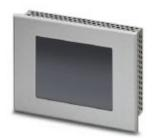
Touch panel with 8,9 cm / 3,5"-FSTN-display (analog resistive (polyester)), 320 x 240 pixel(s) (QVGA), 256-step grayscale, Arm9™, 200 MHz, 2x USB host 2.0, 1 x Ethernet (10/100 Mbps), RJ45, Windows CE 5.0 and user software: TSvisRT. (bus system: PROFIBUS DP)
