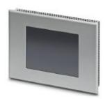
Touch panel with 14.5 cm/5.7" FSTN-display (analog resistive (polyester)),  $320 \times 240$  pixel(s) (QVGA), 5 grayscales, Arm9<sup>™</sup>, 200 MHz, 2x USB host 2.0, 1x COM (RS-232/485), 1 x Ethernet (10/100 Mbps), RJ45, Windows CE 5.0 and user software: TSvisRT. (bus system: without)
