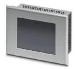
Touch panel with 9.7 cm/3.8" FSTN-display (analog resistive (polyester)), 320 x 240 pixel(s) (QVGA), 5 grayscales, Arm9™, 200 MHz, 2x USB host 2.0, 1 x Ethernet (10/100 Mbps), RJ45, Windows CE 5.0 and user software: TSvisRT. (bus system: PROFIBUS DP)
