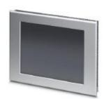
Touch panel with 26.4 cm/10.4" TFT-display (analog resistive (polyester)), 800 x 600 pixel(s) (SVGA), 65536 colors, Arm9 $^{\text{TM}}$ , 200 MHz, 2x USB host 2.0, 1x COM (RS-232/485), 1 x Ethernet (10/100 Mbps), RJ45, Windows CE 5.0 and user software: TSvisRT. (bus system: without)
