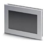
Touch panel with 17.8 cm/7" TFT-display (analog resistive (polyester)), 800 x 480 pixel(s) (WVGA), 262144 colors, Arm<sup>®</sup> Cortex<sup>®</sup>-A8, 800 MHz, 2x USB host 2.0, 1x COM (RS-232), 1x COM (RS-422/485), 1 x Ethernet (10/100 Mbps), RJ45, Windows<sup>®</sup> Embedded Compact 7 and user software: Movicon<sup>™</sup>. (bus system: DualCAN)
