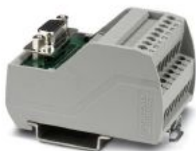
VARIOFACE module, with screw connection and high density D-Subminiature female connector, for mounting on NS 35, no. of pos.: 15, width: 44.9 mm
