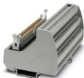
VARIOFACE module, with screw connection and flat-ribbon cable connector, for mounting on NS 35 rails, with pin strip and short and long locking latches for socket strips, 64-pos., with LED
