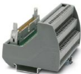
VARIOFACE module, with screw connection and flat-ribbon cable connector, for mounting on NS 35 rails, with pin strip and short and long locking latches for socket strips, 50-pos., with LED
