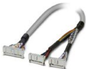
Round cable set; connection 1: IDC/FLK socket strip (1x 20-position); connection 2: IDC/FLK socket strip (2x 14-position); cable length: 1 m
