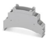
DIN rail housing for use in distribution boards in accordance with DIN 43880, Upper housing part for PCB terminal blocks with screw connection, width: 17.8 mm, height: 89.7 mm, depth: 53.4 mm, color: light gray (7035)
