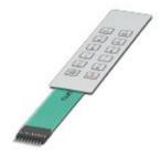
Membrane keypad, self-adhesive, silver conduction technology, 12 keys, embossed, 3 colors, connection cable: 88.5 mm, with crimp female connector RM 2.54 mm, operating temperature -20  $^{\circ}$ C ... 70  $^{\circ}$ C
