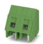
PCB terminal block, nominal current: 17.5 A, rated voltage (III/2): 630 V, nominal cross section: 1.5 mm², pitch: 7.5 mm, number of positions: 5, connection method: Screw connection with tension sleeve, mounting: Wave soldering, conductor/PCB connection direction: 55 °, color: green, Pin layout: Linear pinning, Solder pin [P]: 3.5 mm
