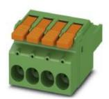
PCB connector, nominal current: 41 A, rated voltage (III/2): 1000 V, nominal cross section: 6 mm², number of positions: 4, pitch: 7.62 mm, connection method: Push-in spring connection, color: green, contact surface: Tin
